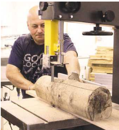
Pic.3 ...to which the board is tacked in order to guide the log while the second face is cut
